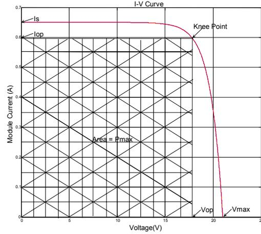
Fig. 2 I-V Curve for a Photovoltaic Module
