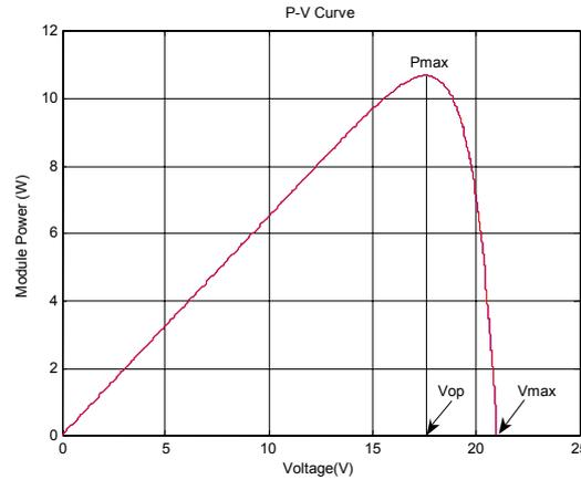
Fig. 3 P-V Curve for a Photovoltaic Module
