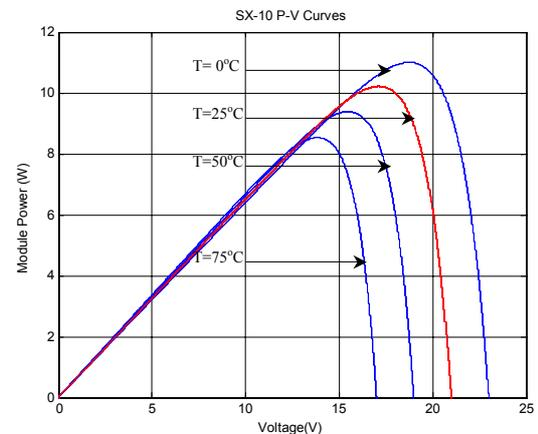
Fig. 6 P-V Curves for the SX-10 module under different temperatures
