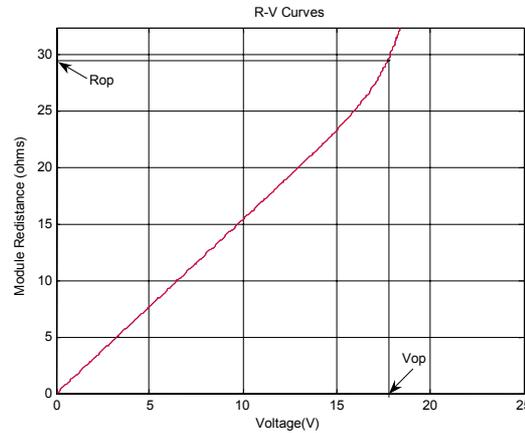
Fig. 4 R-V Curve for a Photovoltaic Module
