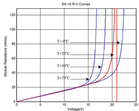
Fig. 7 R-V Curves for the SX-10 module under different temperatures
