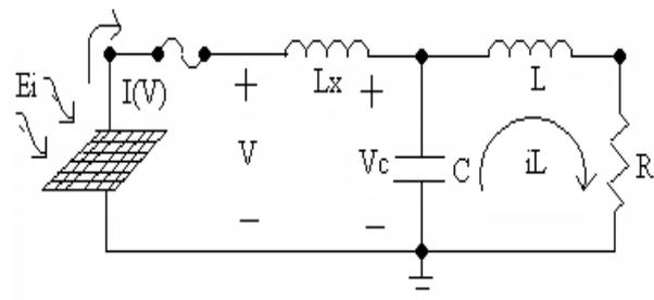
Fig. 1 PV Module Connected to a Transmission Line and a RL Load.
