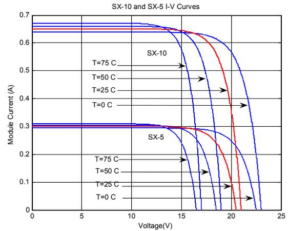
Fig. 5 I-V Curves for the SX-10 and SX-5 under different temperatures
