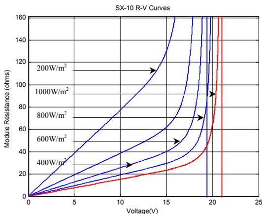
Fig. 10 R-V Curves for the SX-10 module under different effective irradiance levels
