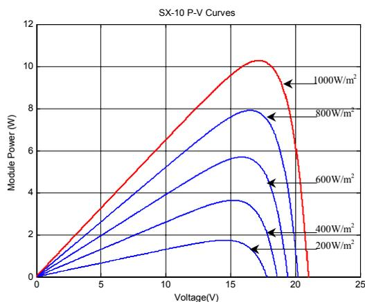
Fig. 9 P-V Curves for the SX-10 module under different effective irradiance levels
