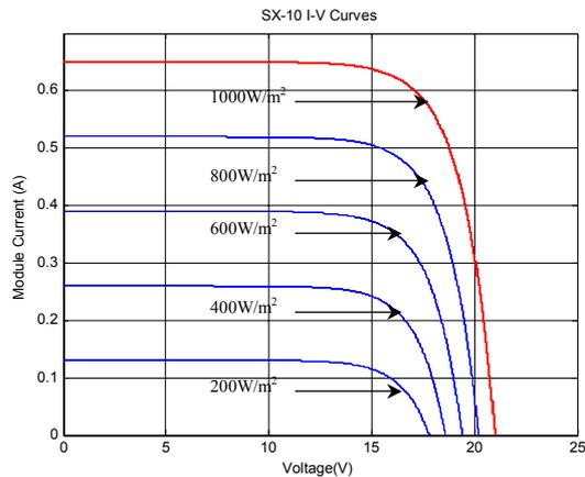
Fig. 8 I-V Curves for the SX-10 and SX-5 modules under different effective irradiance levels
